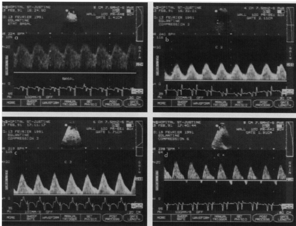
FIG 2. Flow velocity profile through the umbilical artery during basal (panel a) and the last three progressively increasing stages of compression (panels b, c, and d). As shown, a progressive decrease in forward diastolic flow was noted (panels b and c) that ultimately resulted in a brief retrograde diastolic flow during the final level of compression (panel d).
